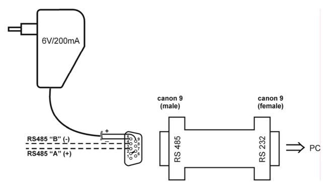
The ATM-AC01 converter is an optional accessory for connection of transmitter/transmitters with RS485 interface to the PC via serial port RS232. Connect connector marked RS232 directly to the PC, connect power to connector marked RS485. Power voltage +6V DC from an external acdc adapter connect to pin 9, 0V connect to pin 5. Also mutually connect pin 2 and pin 7. Link RS485 is connected across pin 3 (A+) and pin 4 (B-).
