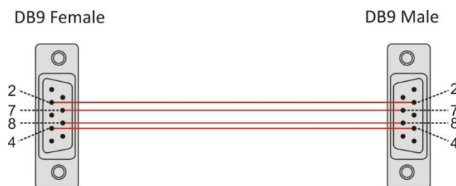
Figure 27 – Building an extension cable
